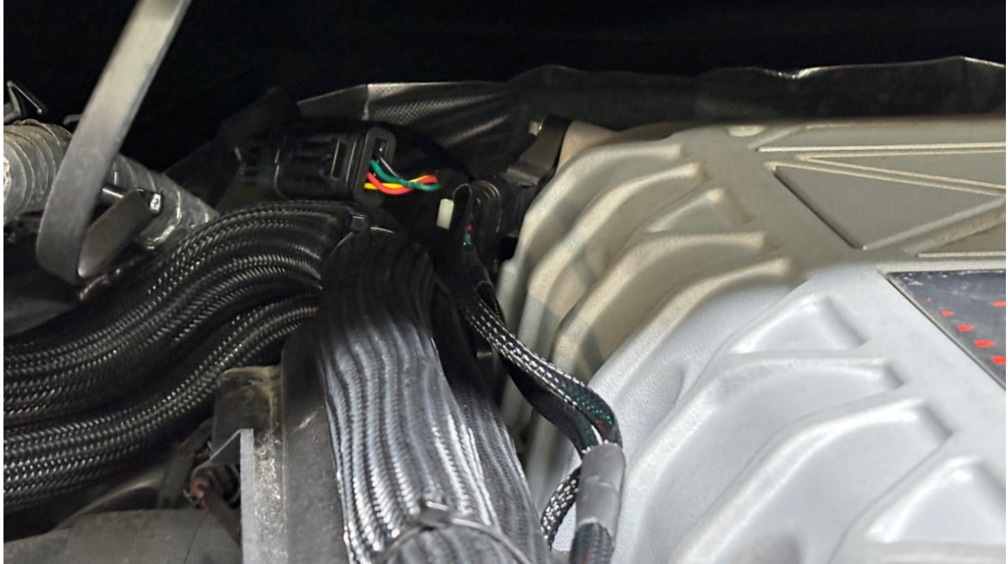
Unplug the TMAP sensor connector by popping out the tab and pinching it and pulling it off. Then plug the JB4 connection in with the brown and black wires into the sensor and then into the factory harness.
