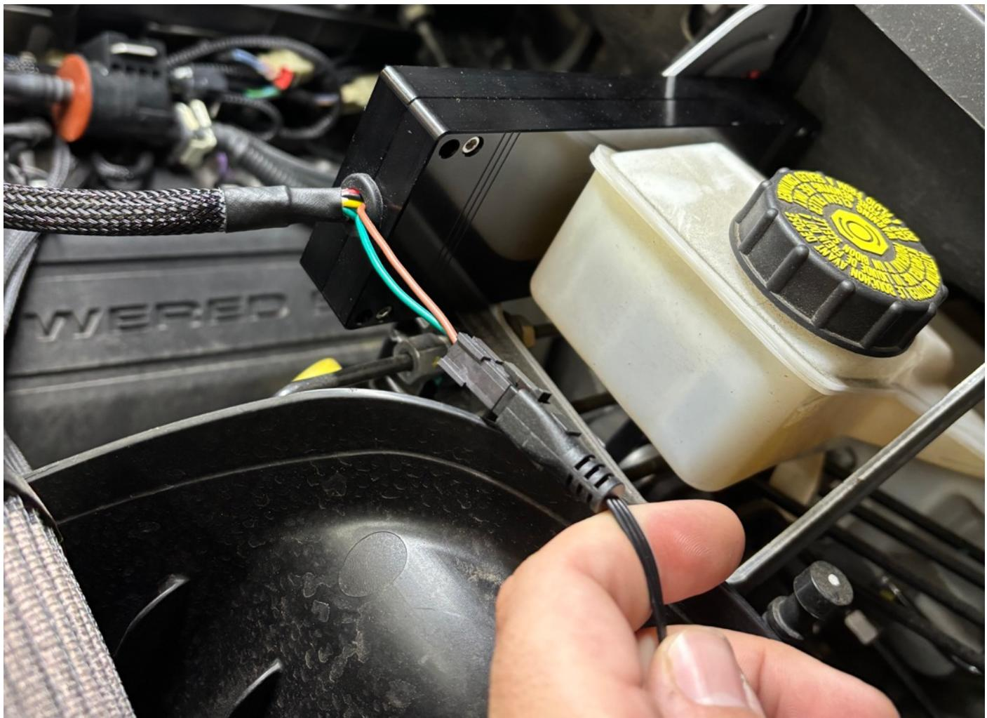
Plug the OBDII into JB4 harness, note correct clip over notch orientation.
