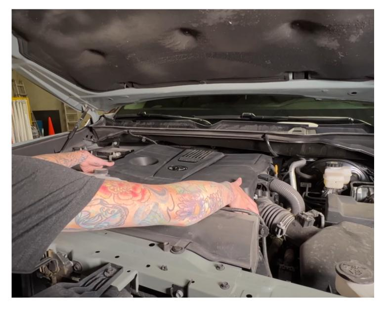
With the ignition switched off and the parking brake set, disconnect the negative battery cable on the battery. Note: Failure to disconnect the battery may cause the CEL to be illuminated upon installation and subsequent operation completion. Do not skip this step! After disconnecting the battery, remove the engine cover.
