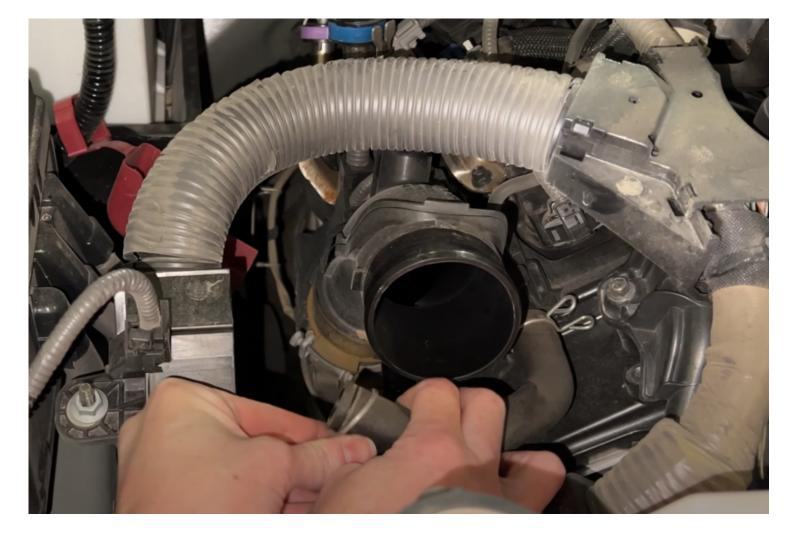
Remove the PCV hose from the intake tube
