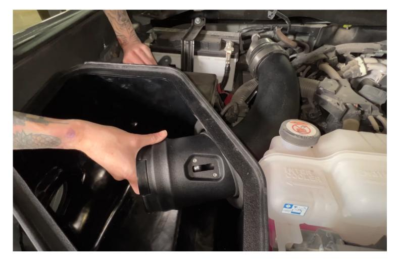
Install the step down coupler onto the intake tube with the head of the hose clamps on the opposite side of the intake tube as the MAF with the clamps facing the passenger side body panel.
