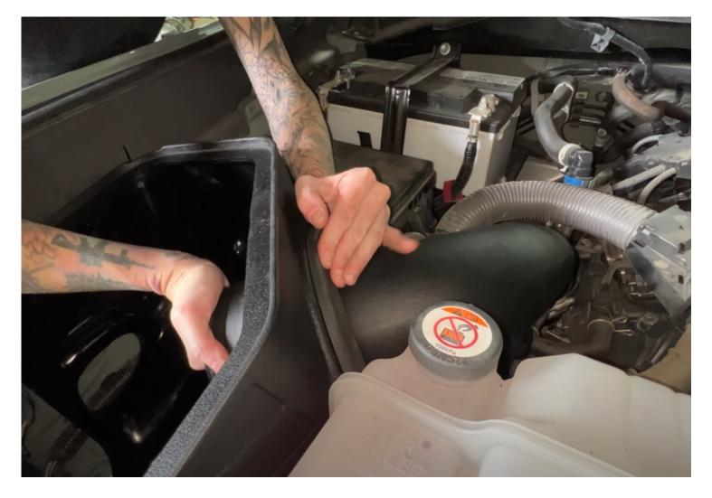
Lift the intake box up and rotate the intake tube onto the turbo inlet.
