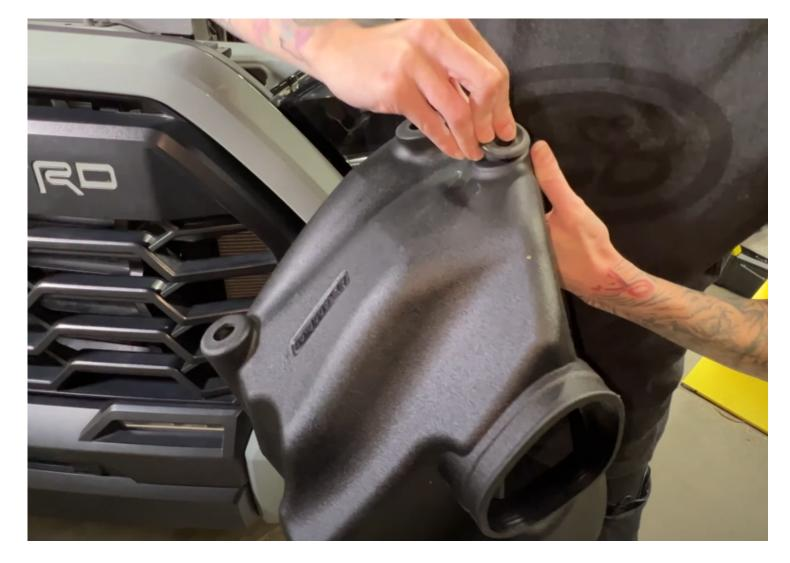
Install 3 grommets into the bottom of the S&B airbox
