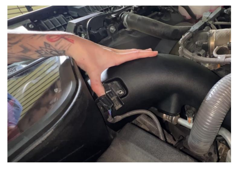
Remove the MAF from the OEM intake tube. Install the MAF gasket (O), MAF mount (T), then use the included screws (P) to install the OEM MAF to the S&B intake. Reconnect the MAF sensor harness.
