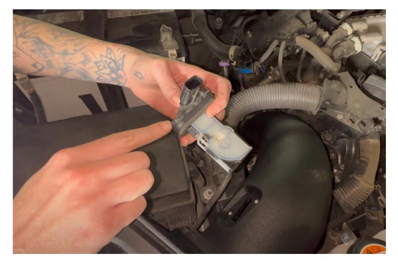
Remove the MAF from the OEM intake and install it onto the S&B intake tube with the MAF gasket (O), MAF mount (T) and included screws (P)
