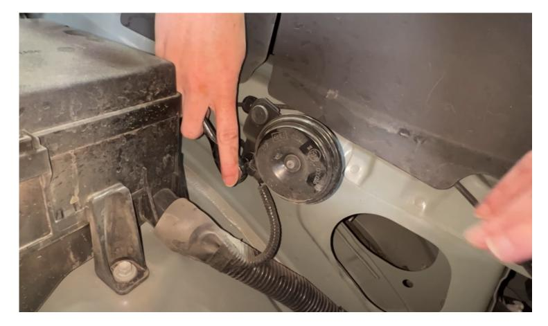
Remove the bolt for the horn to make the install of the intake box easier
