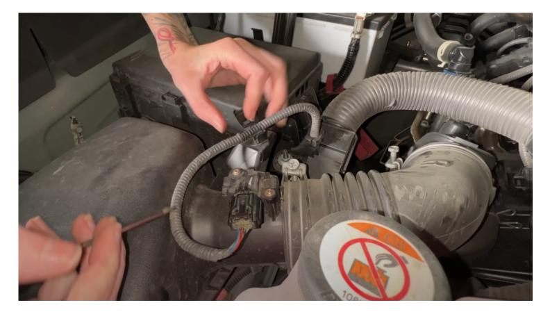
Loosen the bolts, disconnect the clip holding the MAF harness and disconnect the MAF from the OEM intake tube. You can then remove the OEM air box from the truck.
