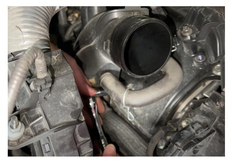
Remove the bolt securing the intake tube. This bolt will be reused. You can now remove the intake tube from the vehicle
