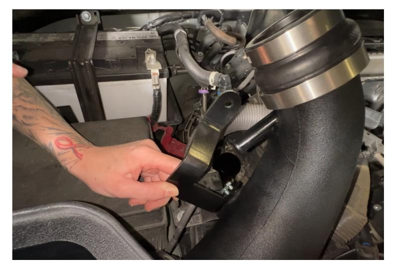
Install the passenger side bracket (K) onto the intake tube with the supplied washers (AB) and hex head bolts (AA).
