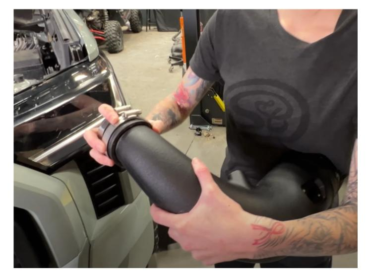
Install the step down coupler(X) onto the intake tube. Please note the direction the hose clamps are pointing. This will make tighten the clamps easier when the tube is installed.
