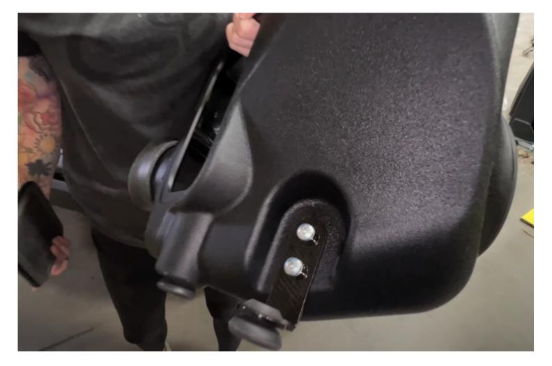
Install the box mounting bracket (U) to the box with the provided hardware and rubber grommets. Install the tube seal and fender seal to the box and install the box plug if you decided to install the box plug on the driver side intake box.
