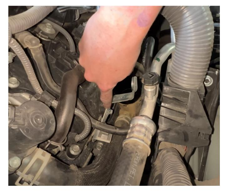
Remove this bolt and put it aside as it will be reused with the S&B mounting bracket
