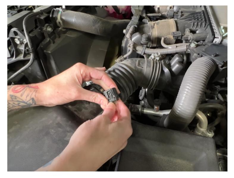
Disconnect the electrical connection to the MAF sensor and loosen two hose clamps (10 mm socket).
