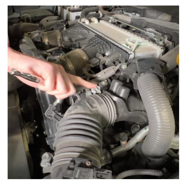
Loosen the bolts for the driver side intake tube
