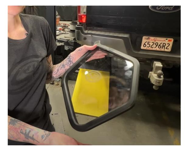
Remove the from the clear lid (E) and install the silicone Lid Seal (F) around the outside edge of the clear lid (E). Then snap into the opening of the airbox
