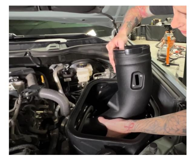
Insert the intake tube through the box and rotate the tube to connect the tube to the turbo inlet.
