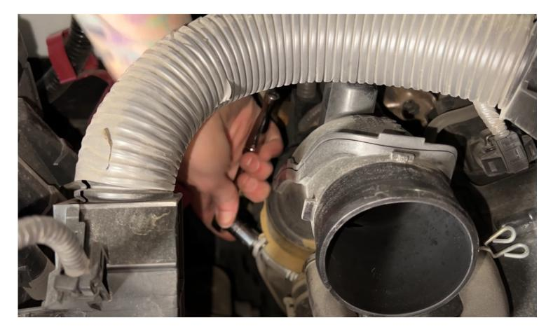
Loosen the hose clamp on the turbo inlet.
