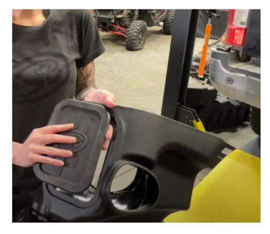
Determine if you want to install box plug (R) to the driver-side box (A). Check the testing results to determine the setup that you desire.
