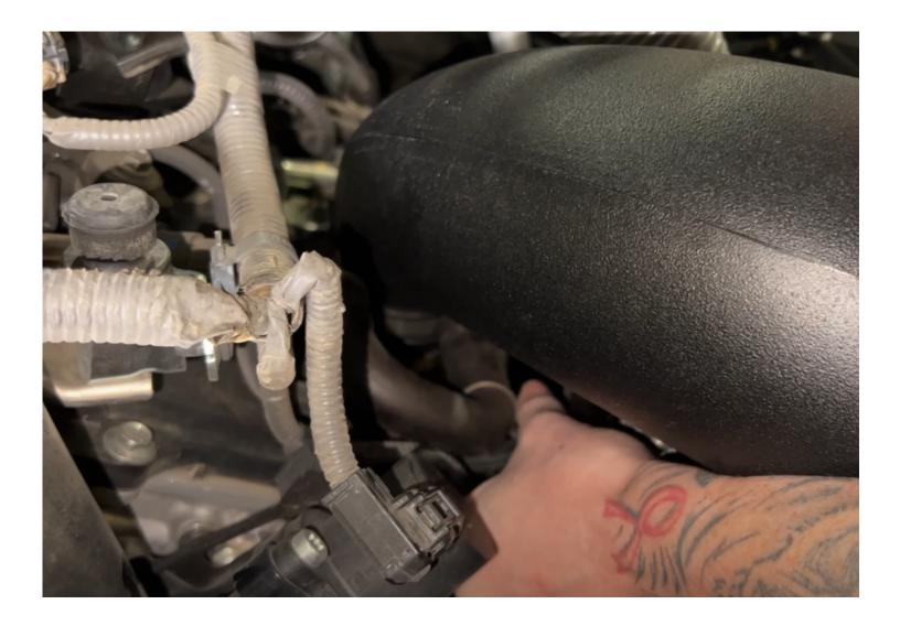
Install the PCV hose onto the S&B intake tube and secure with the clamp. Then use the included hex head bolts(AA) to secure the intake tube to the bracket.
