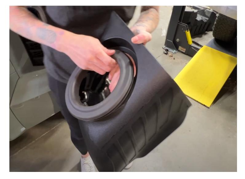
Install the tube seal(Q) and the the fender seal(C) onto the box.
