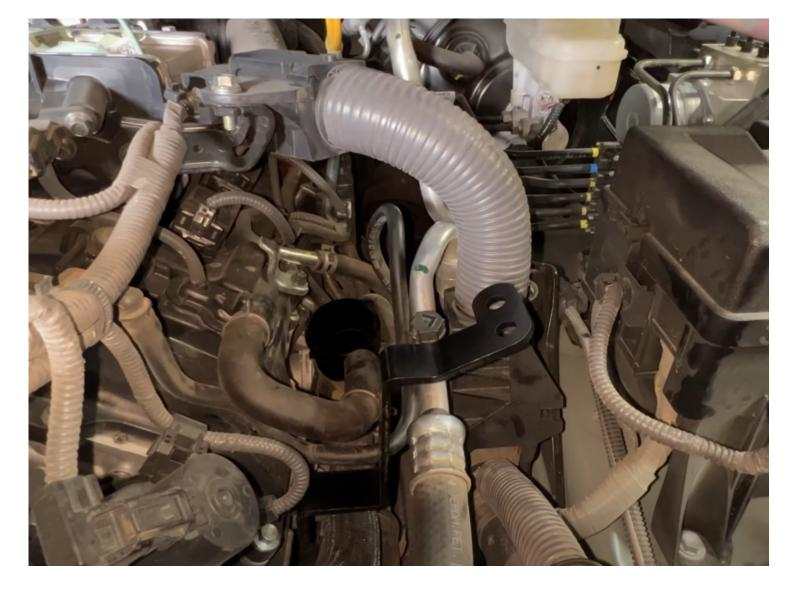
Install the S&B mounting bracket with the bolt you just removed.
