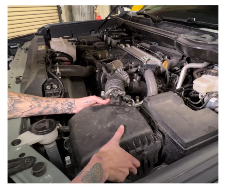
Remove the driver-side Airbox and engine Air intake hose.
