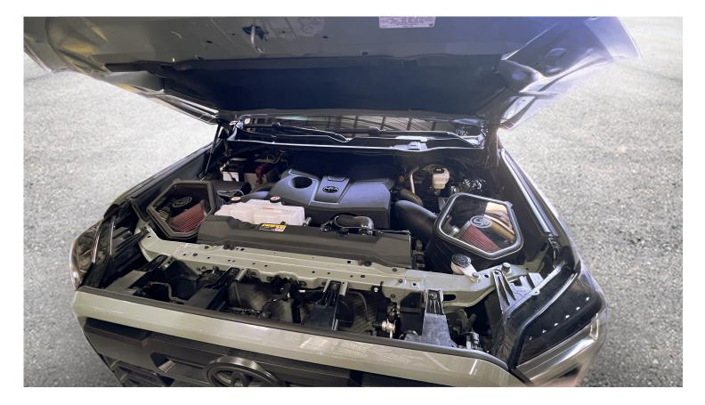
Reinstall the horn on the driver side if you loosened it. Reconnect the battery. Your install is now complete
