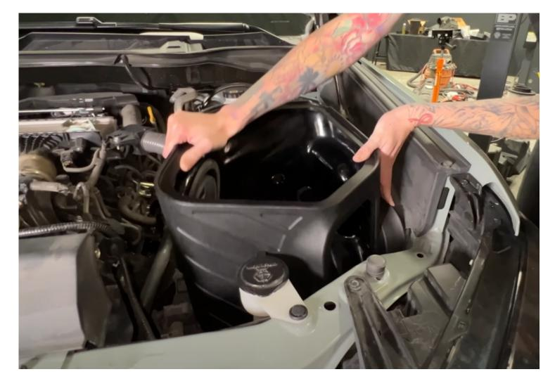
Install the intake box making sure the grommets line up with the body
