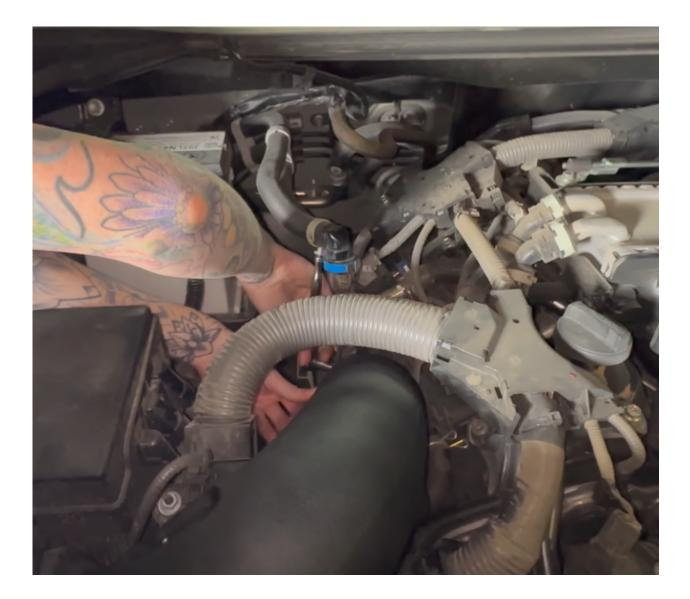
Reconnect the PCV hose to the intake tube, reuse the OEM bolt to secure the bracket to the vehicle and secure the hose clamp on the turbo inlet.
