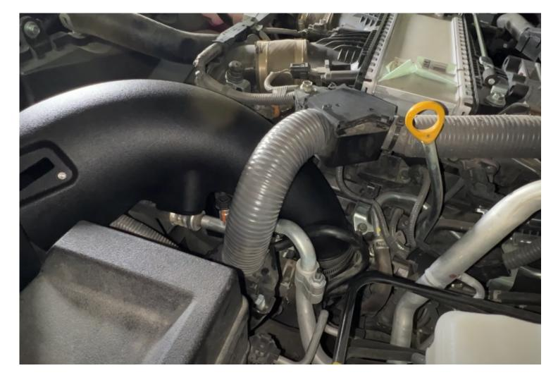
Tighten the hose clamps on the coupler connecting the intake tube to the turbo inlet
