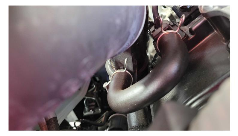
Remove the PCV hose and mounting bolt from the driver-side lower air intake tube.
