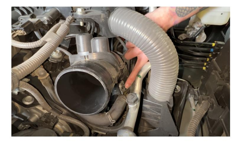
Remove the bolt connecting the OEM mounting bracket to the tube. Keep OEM bracket bolt for S&B Bracket installation. Next loosen the hose clamp connecting the intake tube to the turbo.
