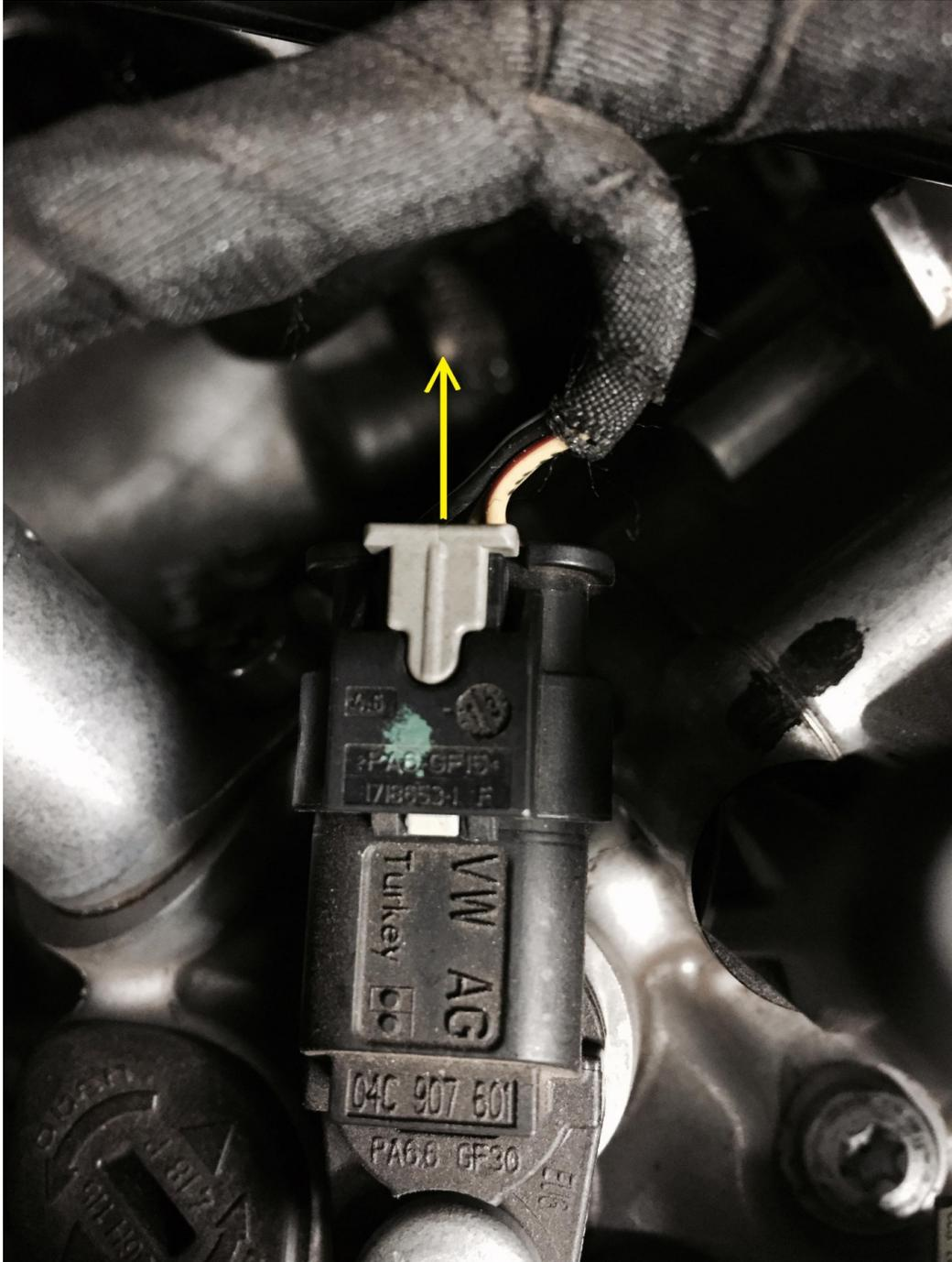
**PLUG B:** The boost sensor plug on the manifold is removed by pushing the grooved tab down on the end of the sensor (yellow square) and pulling the plug towards the back of the car. Plug the removed plug into the male plug on the JB harness and the female plug from the JB harness into the sensor.
