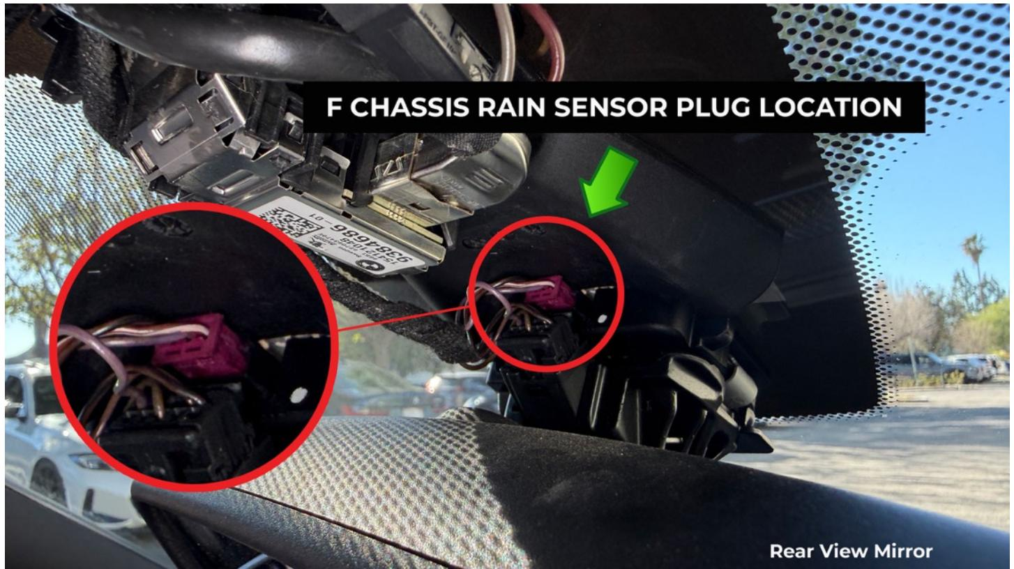
Connect the harness. Make sure they are securely clicked in and replace the 2 halves of the rain sensor cover.
