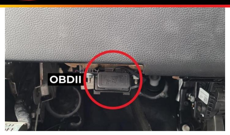
Plug the OBDII wire in to the JB4 green/brown pair connector. If you're able to connect to the JB4 with the app but only see boost and map data, but no other data, then likely the OBDII cable is misaligned, loose, or damaged. Installation is complete! The JB4 comes preset to map1 which is suitable for all 91+ octane fuel. Refer to the map guide within the app or the JB4tech.com JB4 support thread for the platform for the full map guide.
