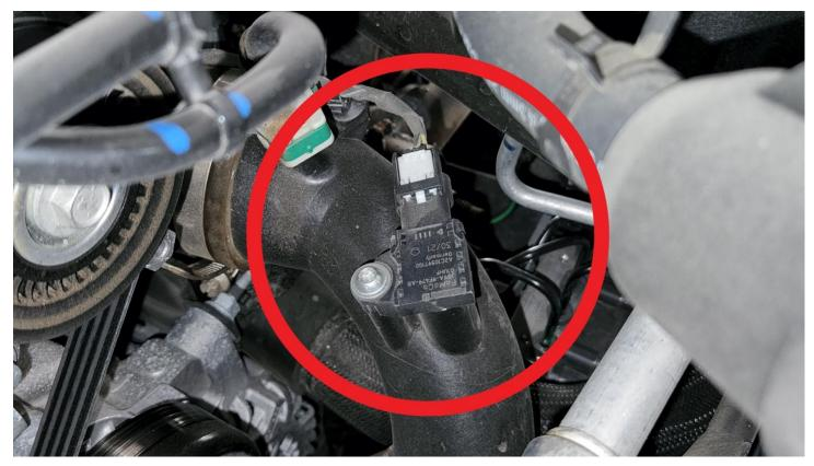
**MAP sensor:** Slide the white clip back and pinch, then pull the connector off to remove. Plug the rainbow colored JB4 wires in here. Then plug the plug from the car into the JB4 wire.
