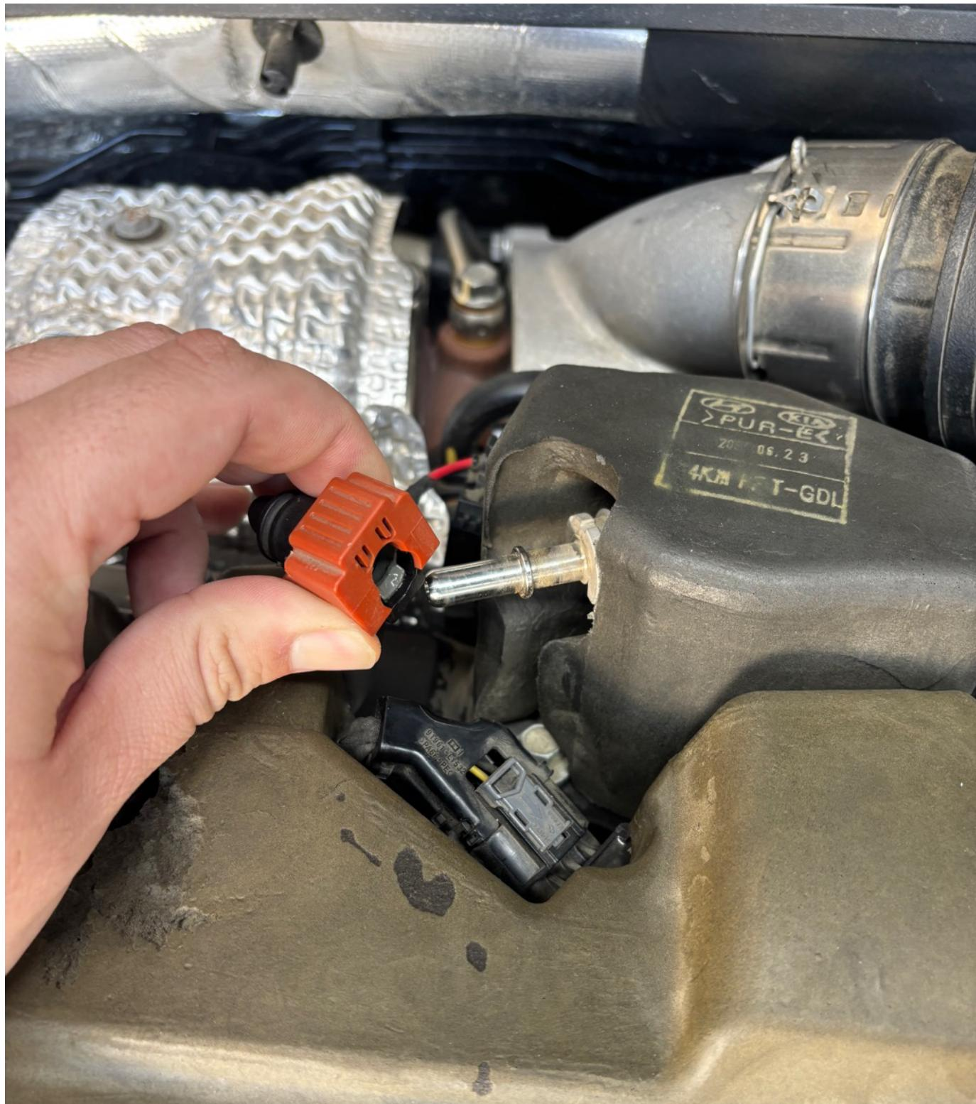
Connect the fuel lines and ethanol content sensor as shown below.
