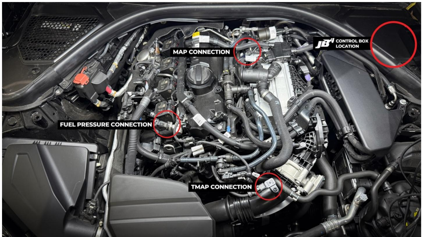
Unplug the TMAP sensor connector by popping out the tab and punching it and pulling it off. Then plug the JB4 connection in with the brown and black wires into the sensor and then into the factory harness.
