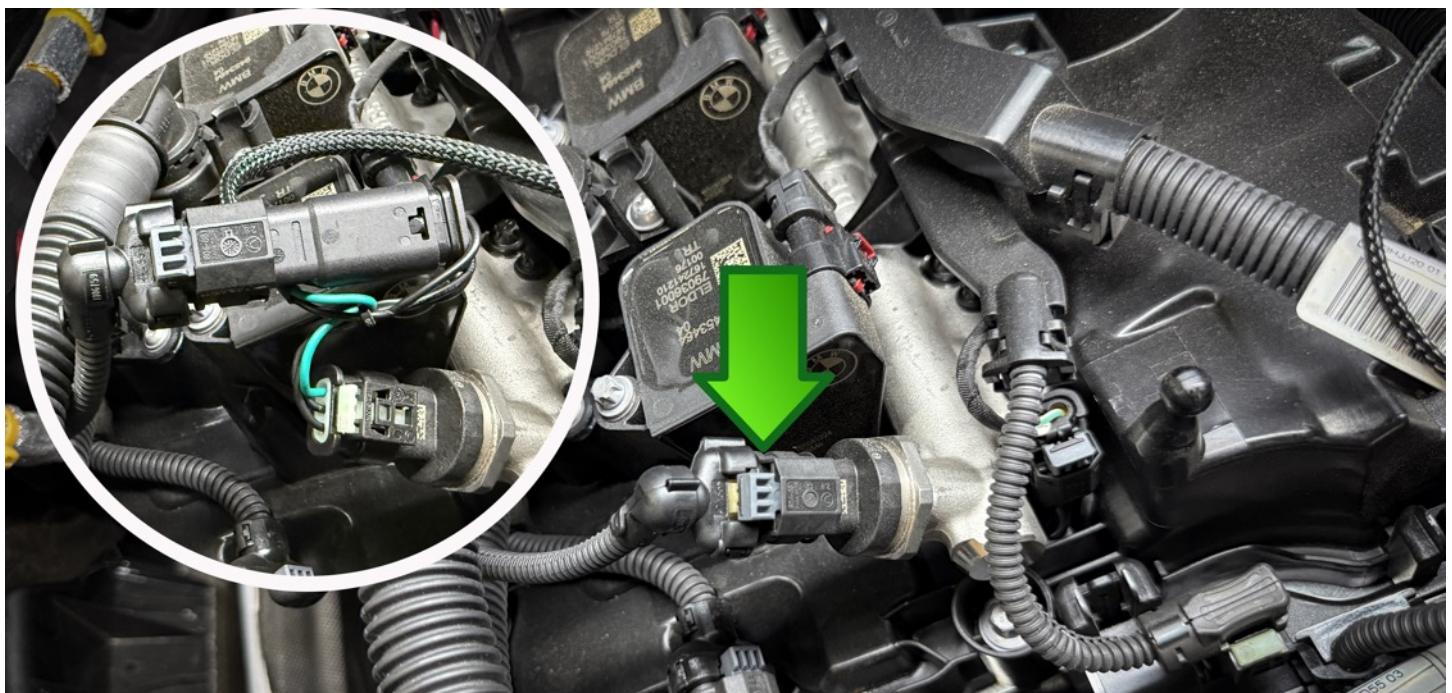
Unplug the MAP sensor connector by popping out the tab and punching it and pulling it off. Then plug the JB4 connection in with the red, yellow, and black wires into the sensor and then into the factory harness.
