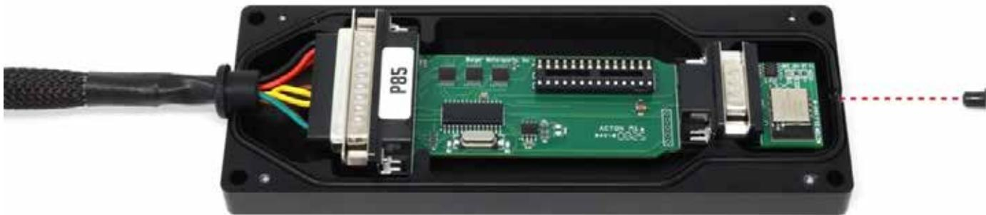
4) Carefully place the top half of the enclosure. When properly aligned it will sit fully flush with the bottom half. If it's not flush, adjust the board position internally. Tightening down the screws when the board is not properly aligned may damage the JB4 control board.
