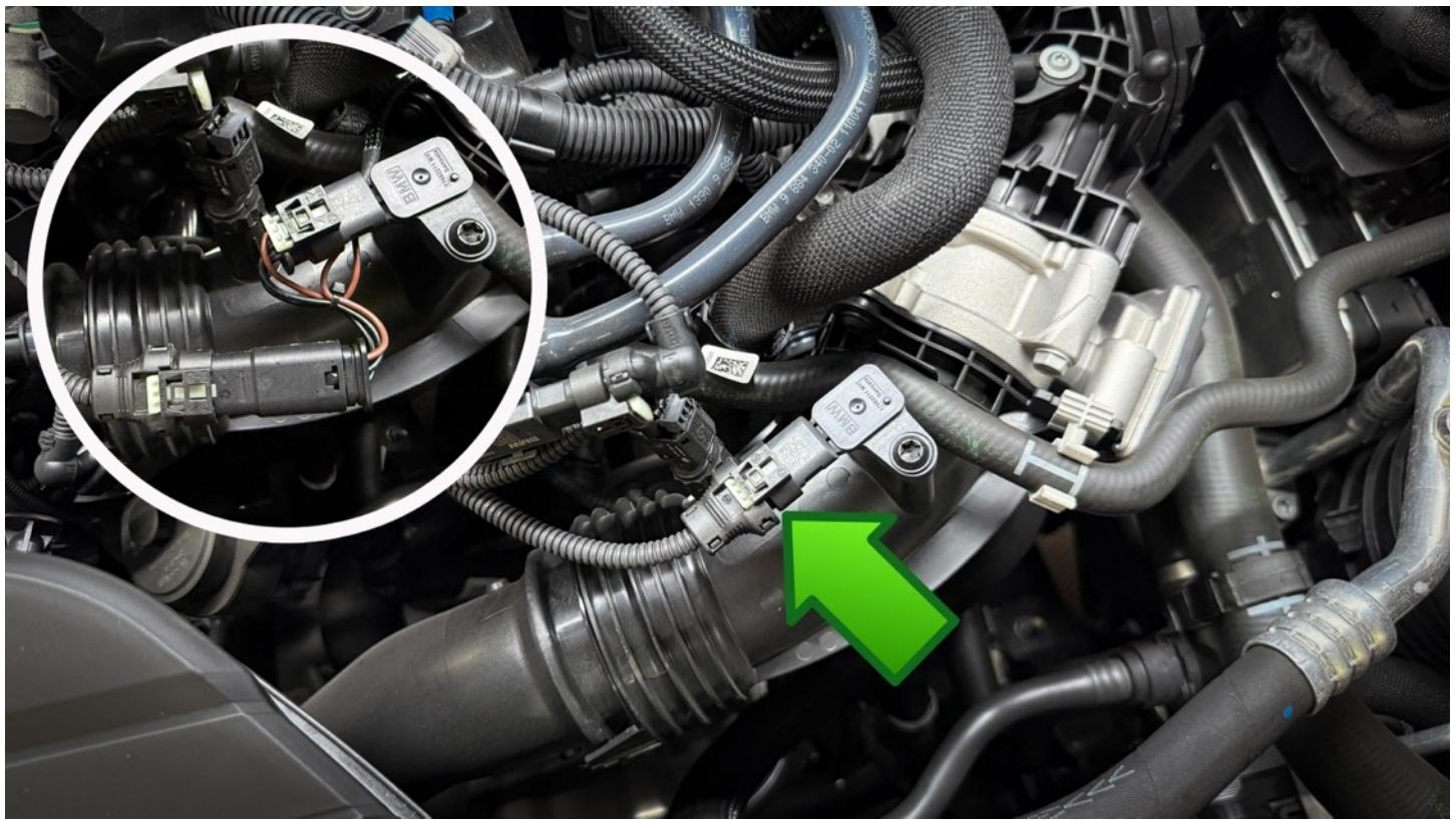
Unplug the fuel pressure sensor connector by popping out the gray tab and punching it and pulling it off. Then plug the JB4 connection in with the green and black wires into the sensor and then into the factory harness.
