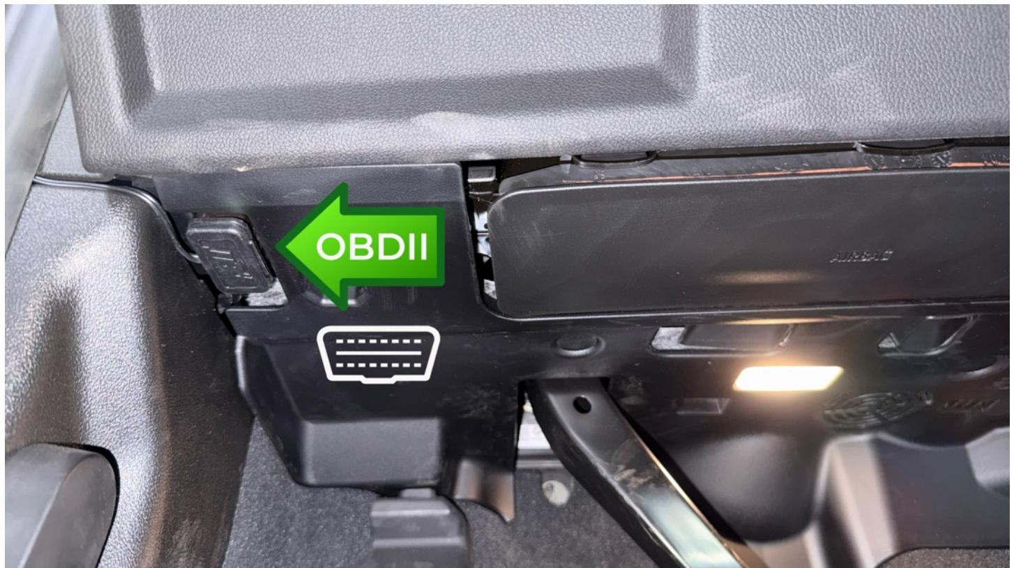
Finally plug OBDII into JB4 harness, note correct clip over notch orientation. If no data appears in JB4 app once connected an issue with the OBDII connection is usually the culprit.
