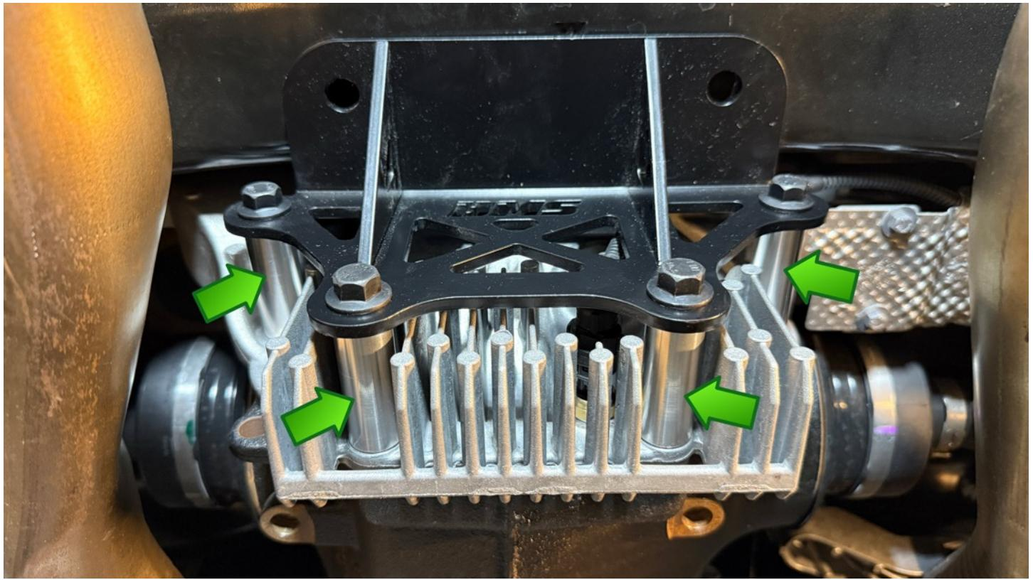
Use a  $\frac{1}{2}$ " drill bit and drill the holes all the way through the top and bottom of the subframe. Make sure the drilled holes are horizontally level. A long drill bit will be needed to drill with the brace on. For shorter bits the brace can be removed and the holes drilled.
