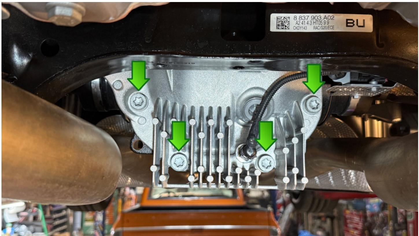
For the 2020-2026 Toyota Supra, remove the damper weight using an E14 socket along with the threaded tab inside the subframe and put these aside. They are no longer needed with the diff brace in place.
