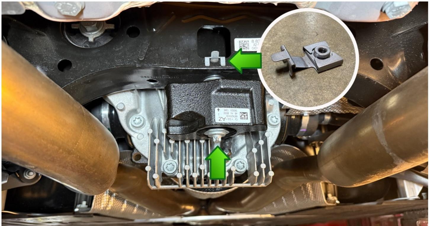
Put the 4 billet spacers between the BMS diff braces and screw them in with the supplied bolts. The two holes below the subframe will be used as templates for the required  $\frac{1}{2}$ " drill holes.
