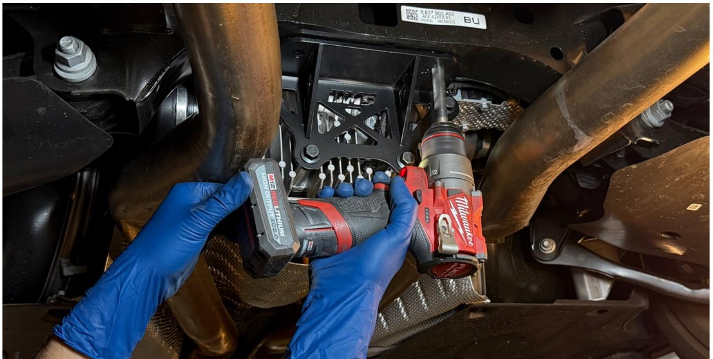
Next place the long bolts through the subframe with the washers and bolts shown in the position below. Double check all the nuts and bolts are tight.
