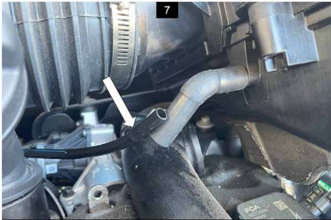
Pull the hard vacuum line out of the rubber hose on the left side of the airbox.
