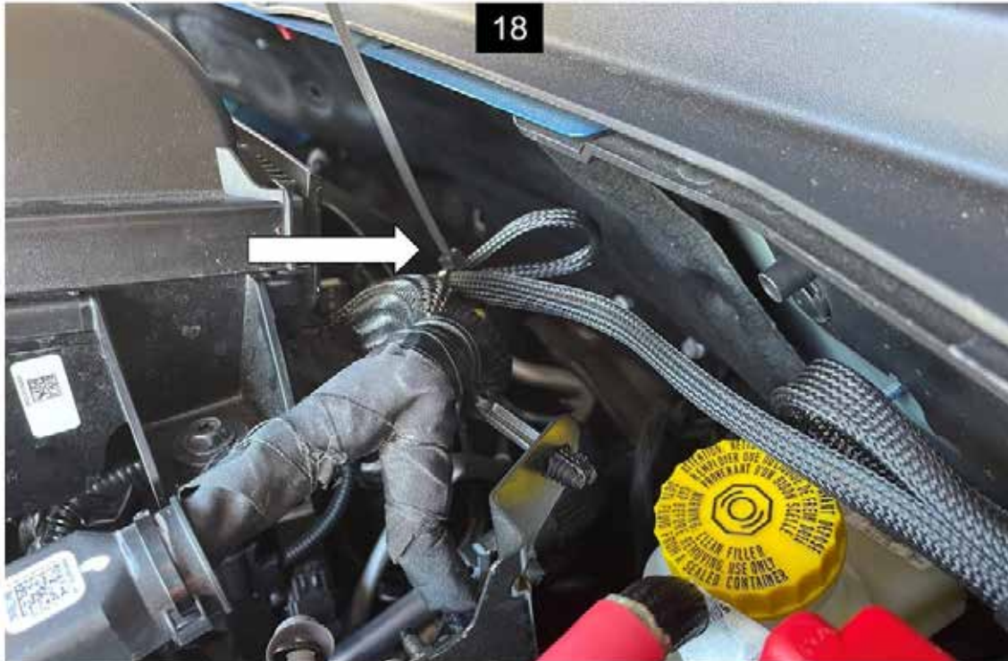
Remove most of the slack from the JB4 wiring harness and secure it out of the way with cable ties
