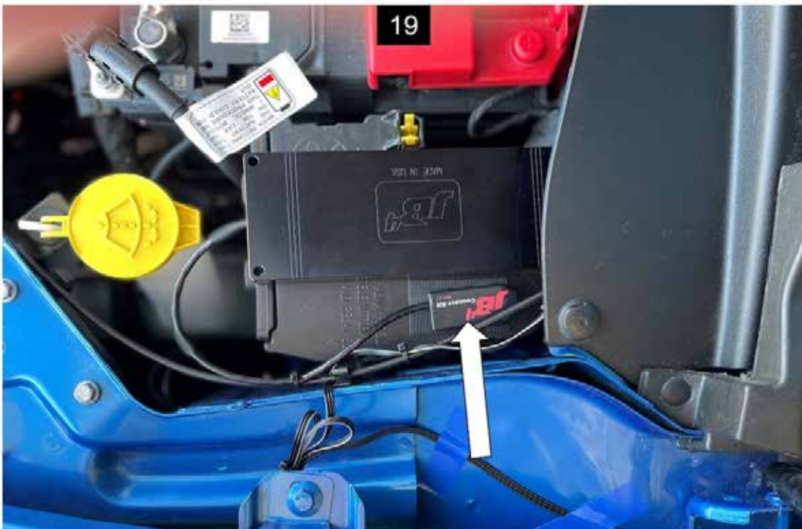
Mount the JB4 unit on top of the fuse box lid, I used heavy duty Velcro. The mobile kit is mounted next to the JB4 unit with Velcro.
