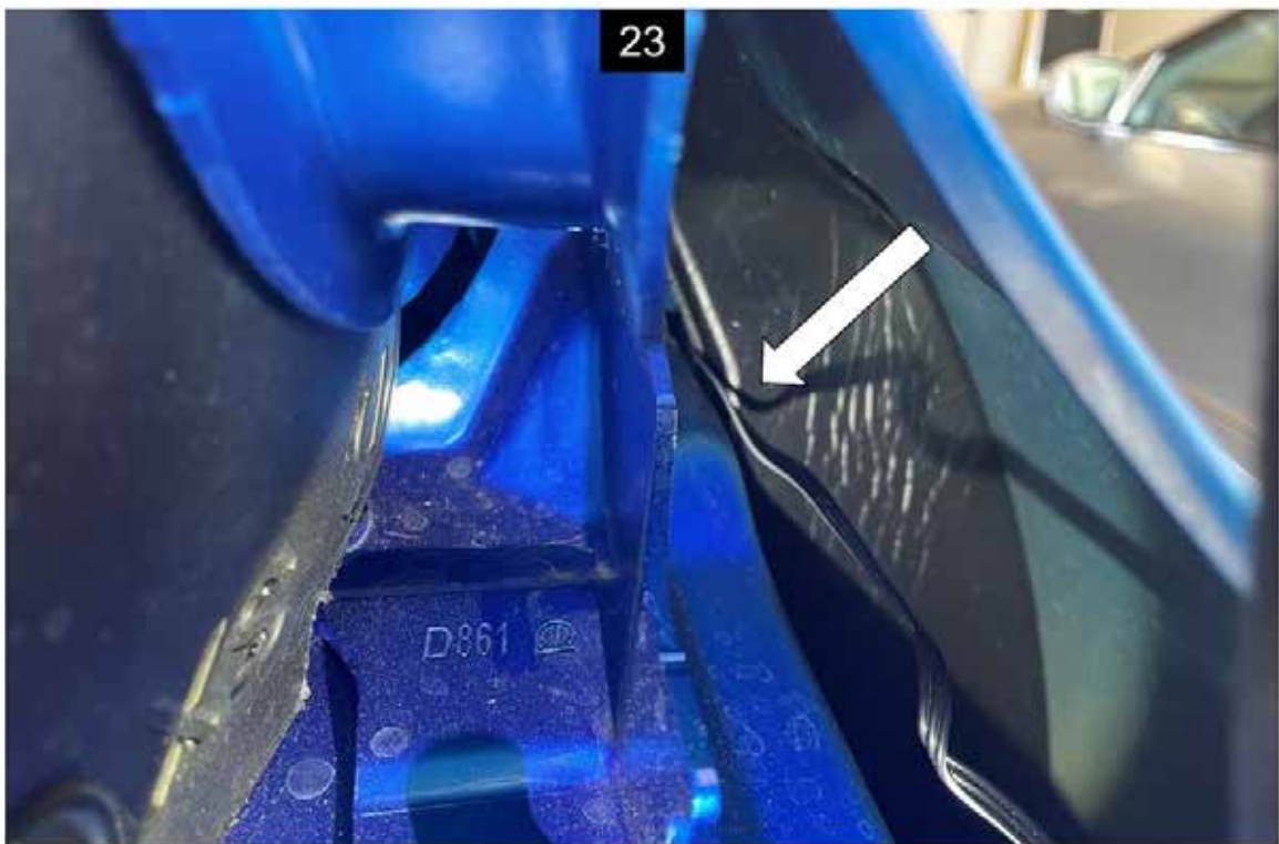
I pushed this foam forward enough to be able to pull the wire from the cabin along the side of the foam using a bent coat hanger.
