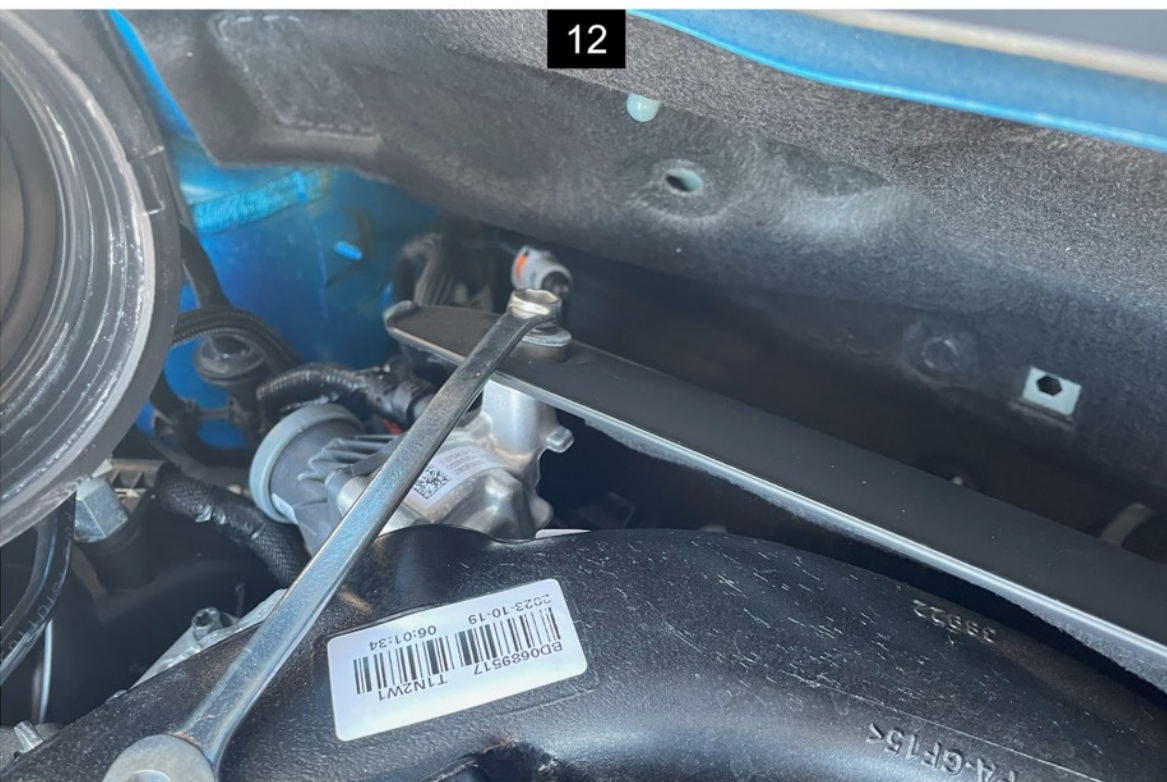
Remove the other 10mm bolt holding the plastic guard to the engine. Push the guard out of the way towards the firewall.
