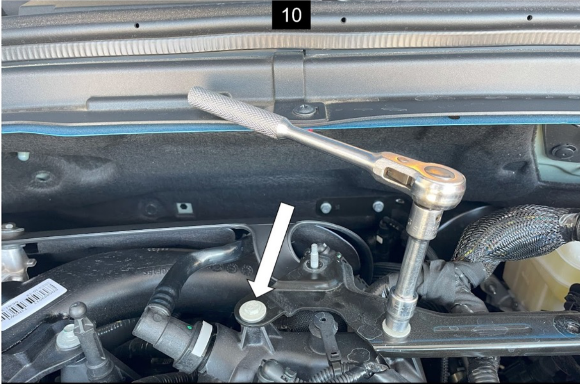
Remove the two 10mm bolts holding the airbox mount to the engine.
