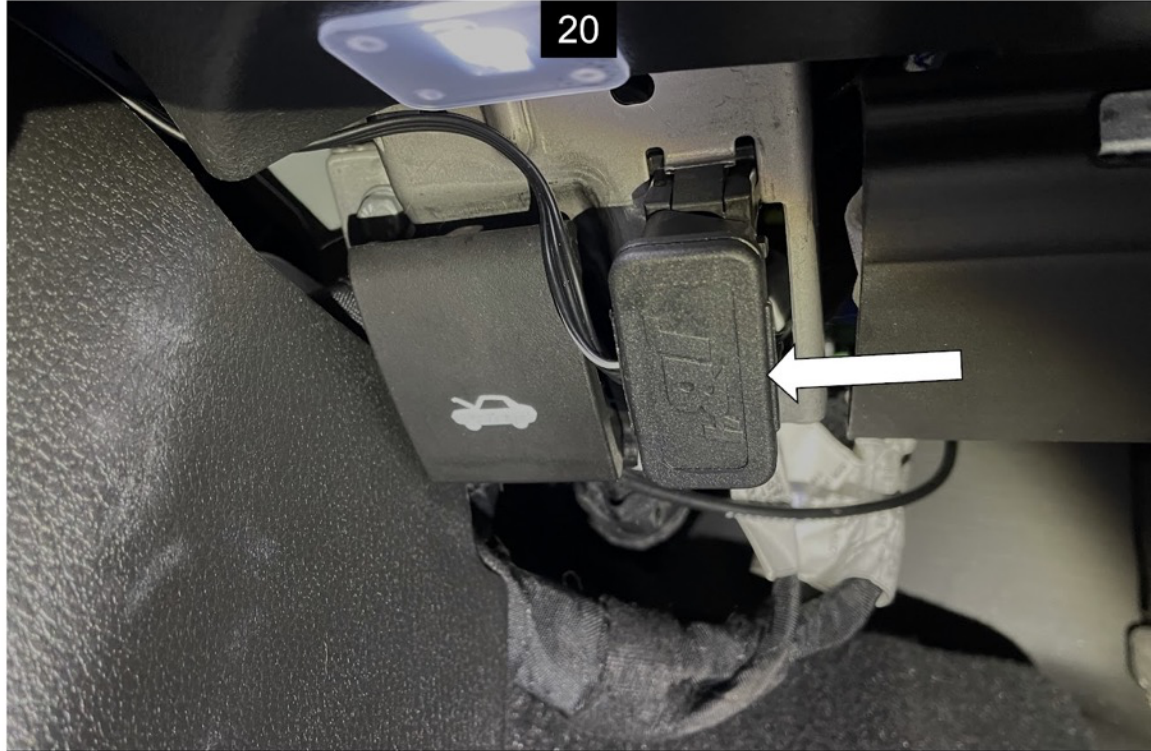
Plug the OBDII unit into the port under the dash next to the driver's door.
