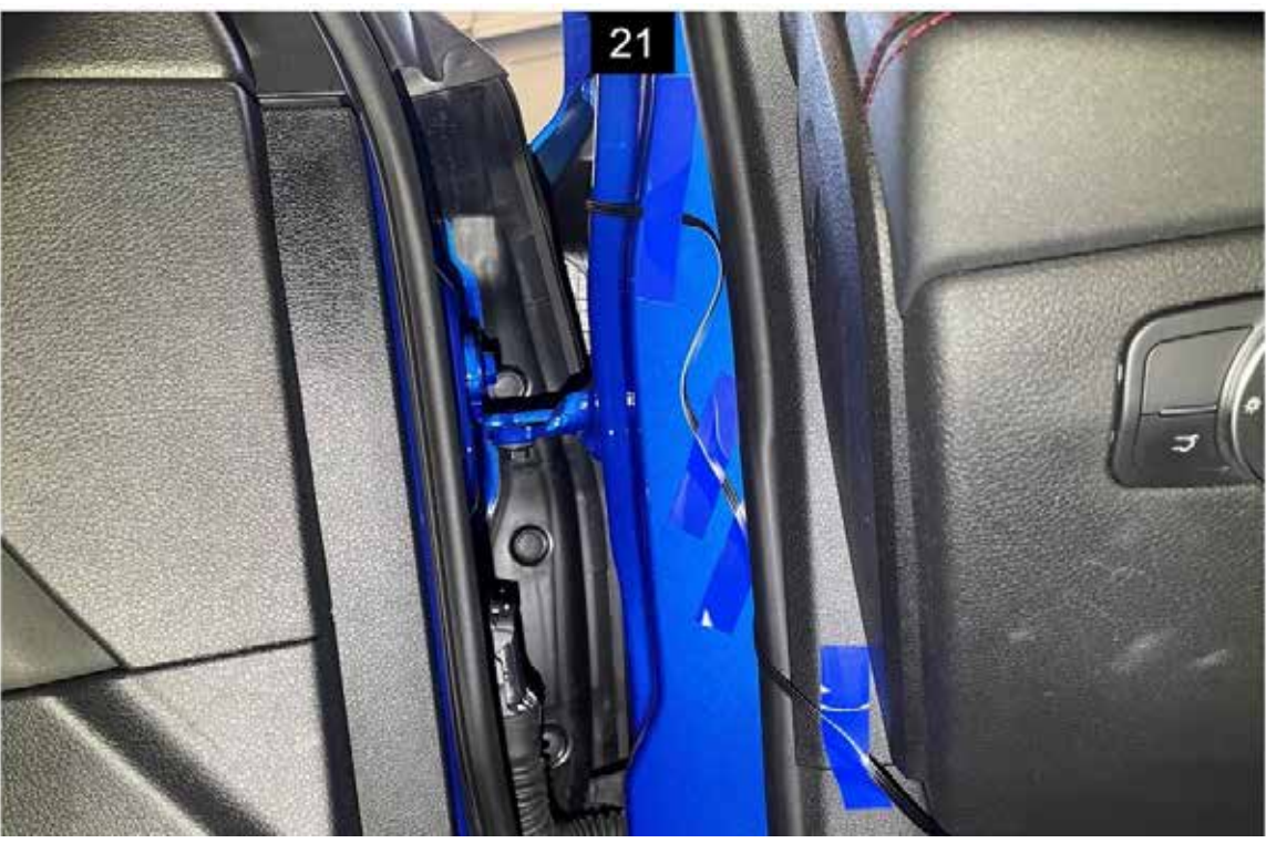
Plug the OBDII unit into the port under the dash next to the driver's door.
