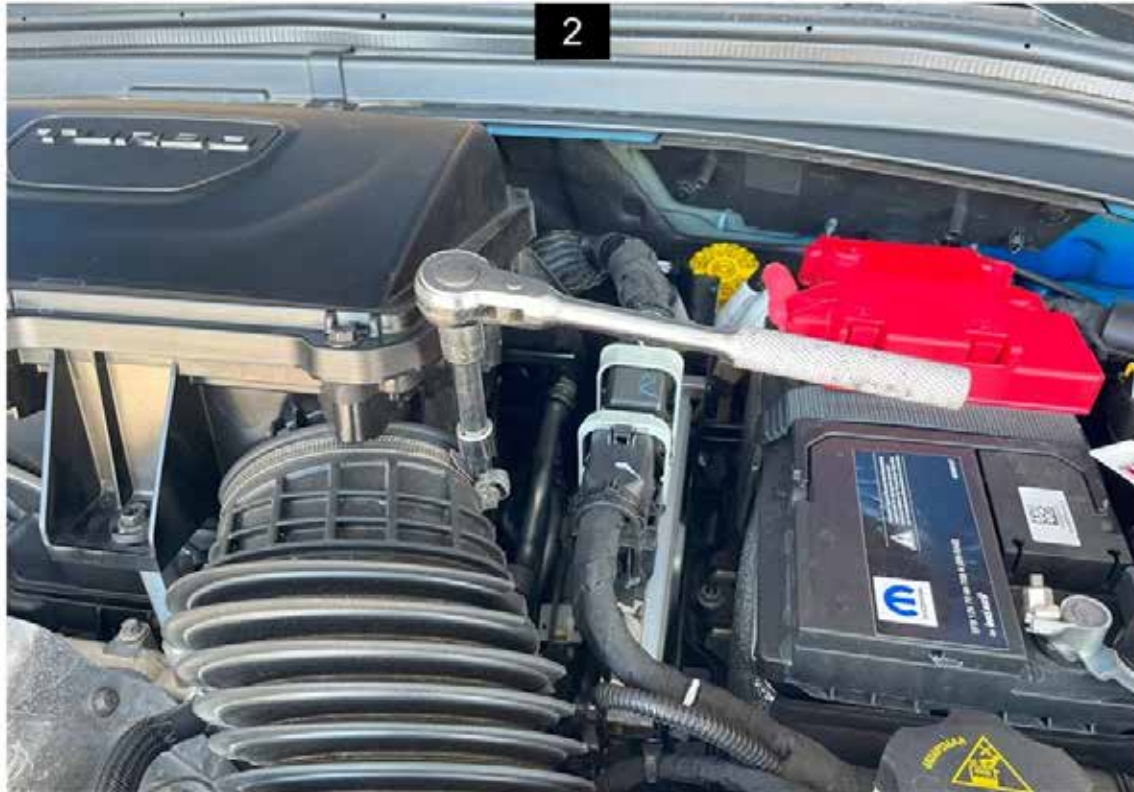
Begin by loosening the airbox inlet hose clamp with a 7mm socket
