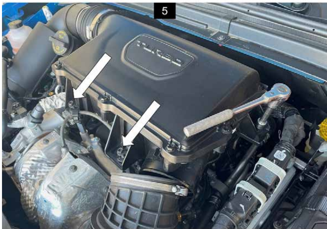
Remove the three 10mm bolts holding the airbox to the engine.
