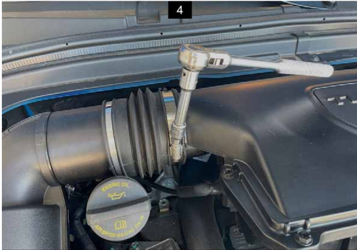
Loosen the airbox outlet hose clamp with an 8mm socket.
