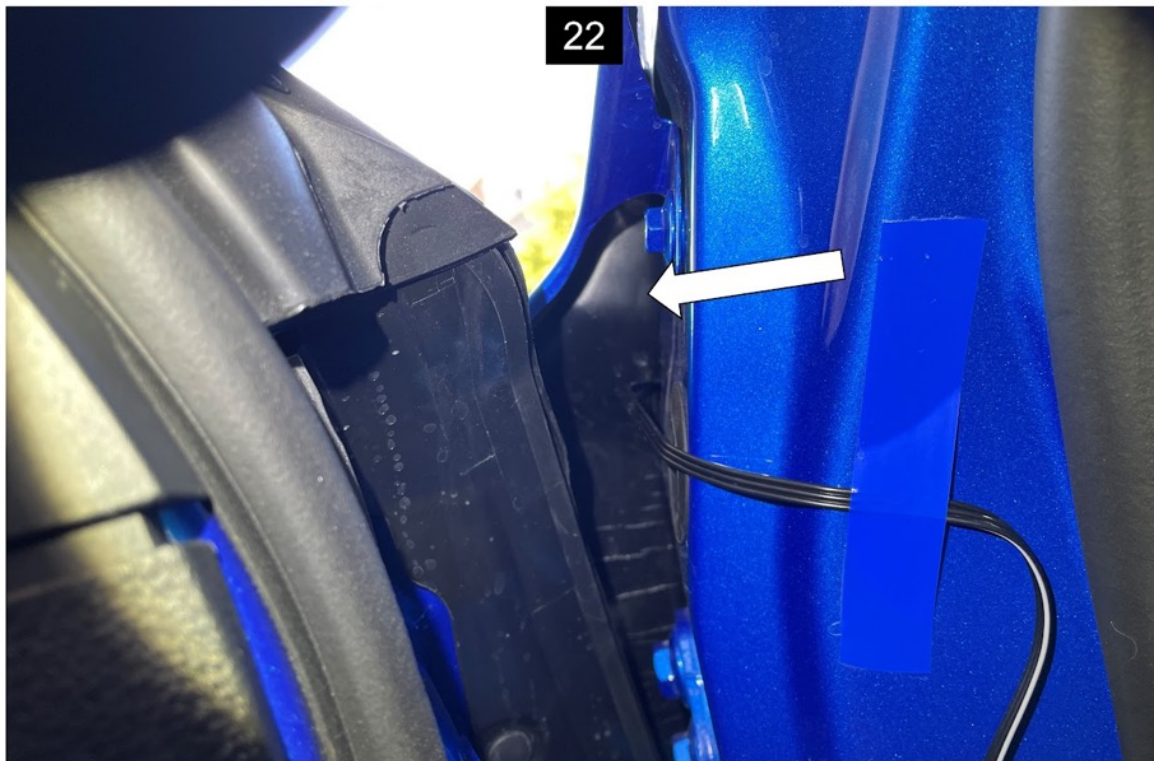
With the driver's door open you can see a black closed-cell foam plug sealing the rear of the engine compartment.
