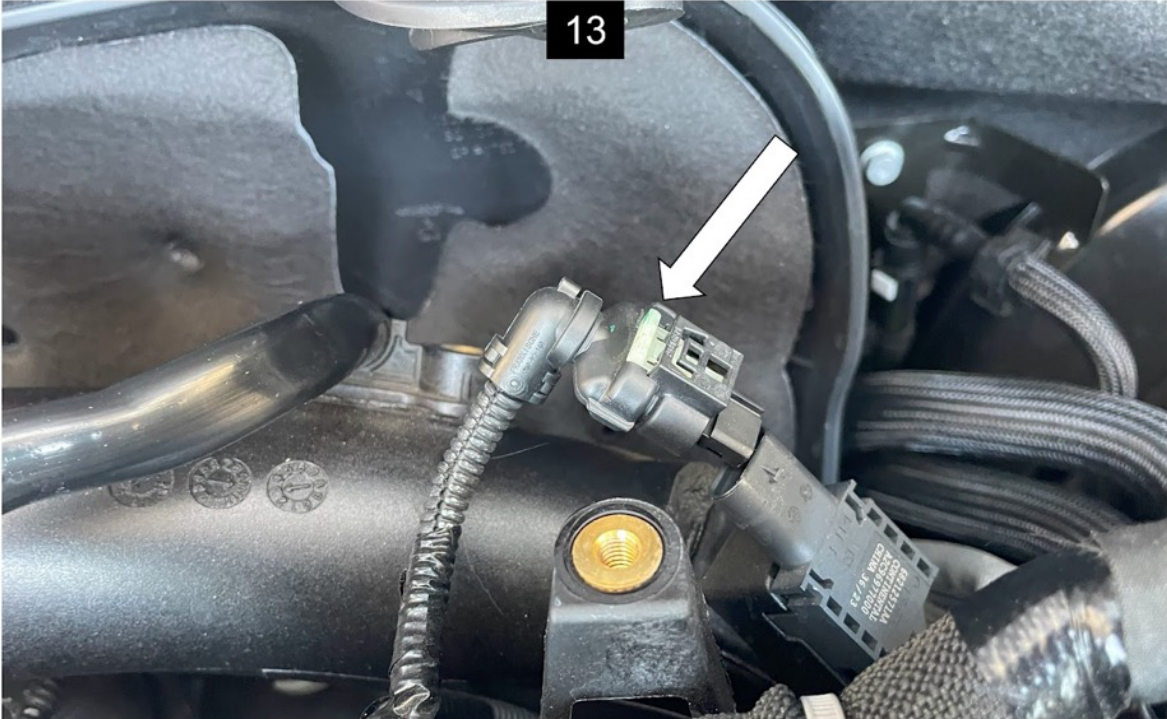
Release the boost sensor plug by pushing the white locking tab towards the factory wiring harness, pressing down on the tab and pulling the plug away from the sensor.
