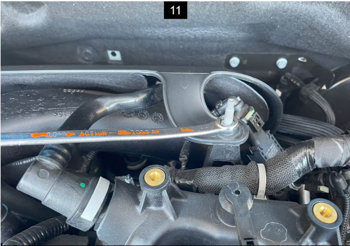
Remove the stud with a 10mm wrench.
