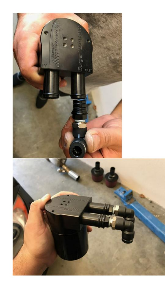
Install the OCC to the strut brace with the included bracket. Note photo below shows our optional boost side OCC. They mount next to each other if equipped with both.
