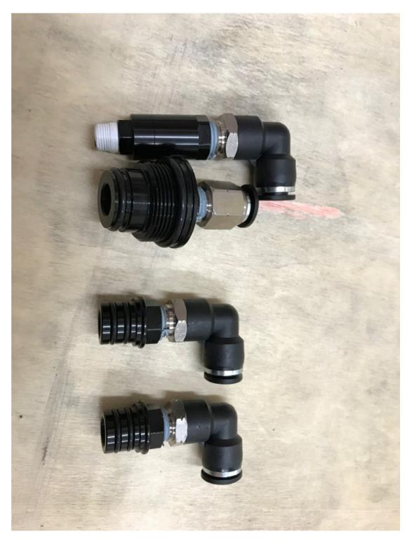
Lube up the O rings on the OCC fittings and insert them in to the OCC bungs.
