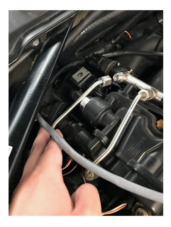
Once removed remove the stock N54 PCV system and internals. Install the OCC fitting onto the valve cover which replaces the factory PCV.
