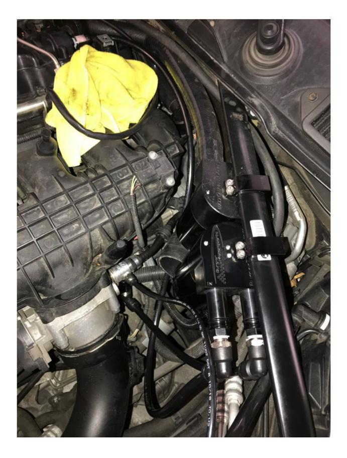
Make sure all push lock tubes are fully pushed and seated in. A little tug will ensure they're in correctly. Install the intakes and engine cover and installation is complete!
