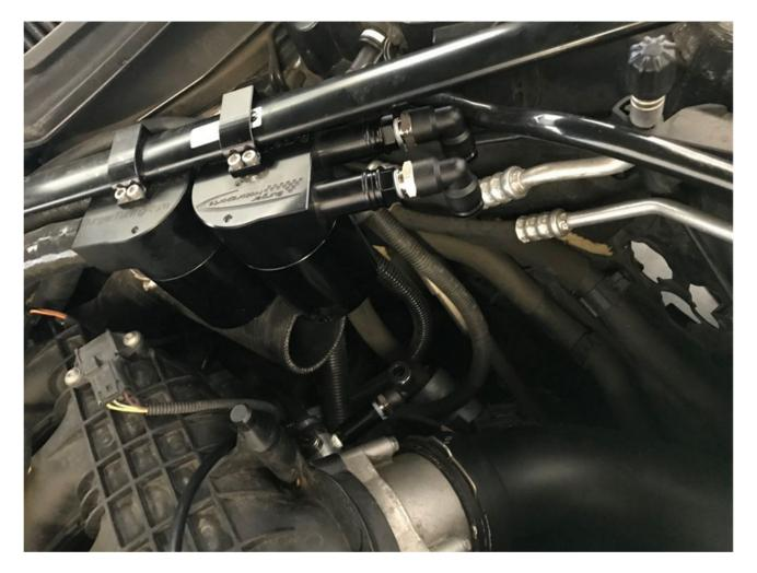
Remove the engine cover to access the PCV valve and if needed remove the rear most high pressure fuel line for additional space. Fuel will spill out of this fitting so have a shop towel ready.
