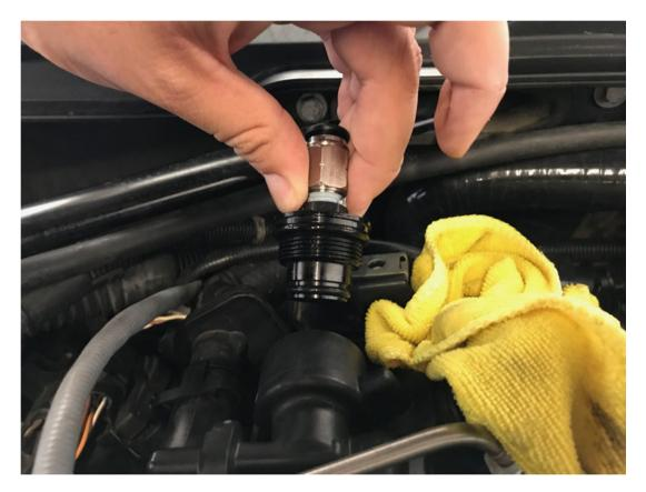
Install the provided push lock tubing. Valve cover tube will be about 34" long and goes to the "IN" on the OCC can. The tube from the check valve will be about 12" long and will go to the "OUT" on the OCC can.
