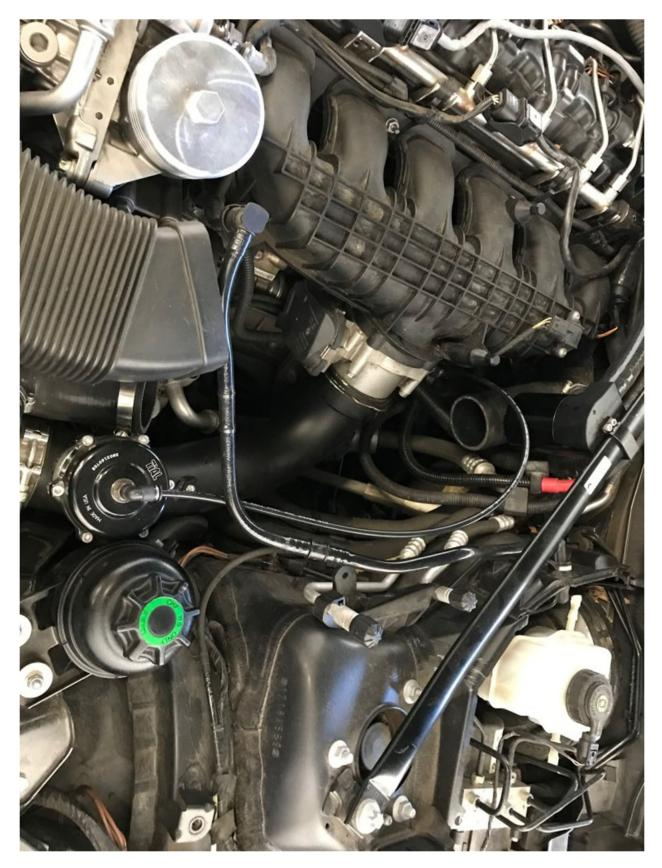
Install the BMS BOV adapter onto the throttle body. Remove the brake boost line by pinching on the tabs and pulling to release. Once moved out of the way, insert the BOV adapter onto the throttle body and lock the E clip into place. Add teflon tape or paste to the 1/8" NPT check valve fitting and tighten in to the BOV adapter. If not equipped with a BOV install the block off cap on the 2<sup>nd</sup> 1/8" NPT fitting.
