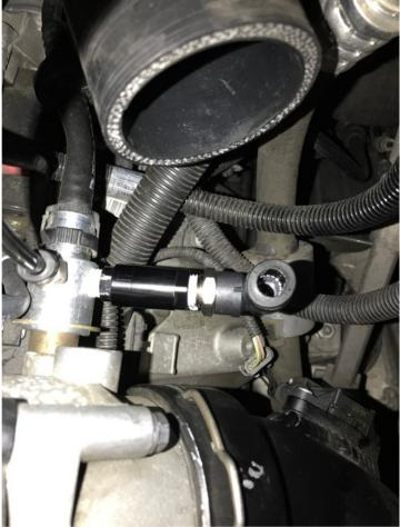
Tighten the quick connect fittings in to the adapters as shown below, note the quick connect fittings come with Teflon tape pre-applied.
